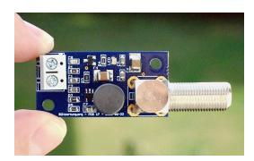
At PCB 20.1 and subsequent boards the free board space at PCB 20.x next to PCB 17.x is used as an experimental electrical antenna. This antenna is designed only for testing purposes. You can also break off this aerial and connect a wire antenna at the two pin header. The external connection point is ground, the central connection point is the antenna. Note that any electrical antenna must be placed outside far away from from buildings and electrical interference sources.
