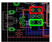
At switch S1 on PCB 19.2 you have to connect pin 5 and pin 6 by a jumper. This turns the board on, if an USB power supply is connected, the red rectangle in the image above. You have also to connect pin 1 and pin 2 by a jumper such that the pre-amplifiers get power, the green rectangle in the image above. Note that these jumper settings are different at the early board PCB 19.1. Please refer to the circuit diagrams.
